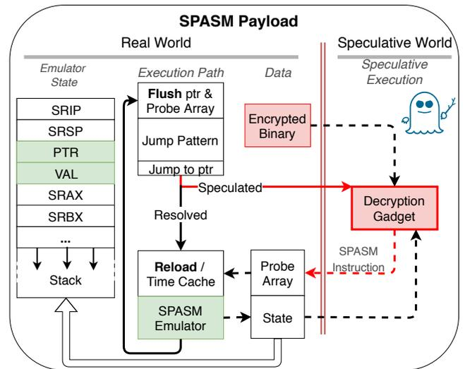
Fig. 9. **SPASM model**—Our SPASM emulator speculatively decrypts instructions, and emulates them in the real world. The *Speculative Computation* decrypts the encrypted SPASM binary using AES, returning the result through the side channel to allow the *Real World* to update the emulated state and make system calls on behalf of the speculative world.
