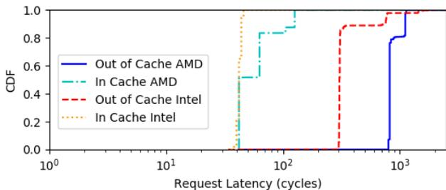
Fig. 2. **Cache latency**— Cumulative distribution function of the cache hit and miss latency for an Intel Xeon-1270 and AMD Epyc 7251. If a cache miss is used to force CPU speculation, the CPU must wait at least 300-800 cycles before the speculated branch can be resolved. However, we find the CPU is occasionally limited to far fewer instructions speculatively, suggesting another limit is at play.
