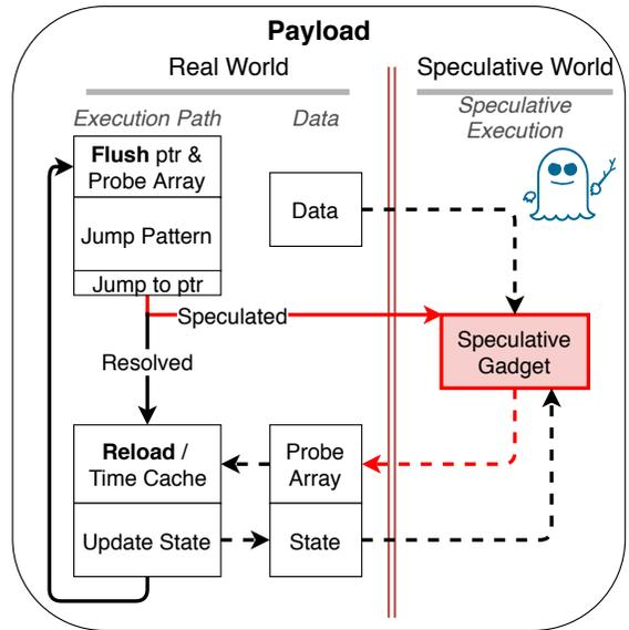
Fig. 5. **ExSpectre model** — General model of speculative computation within the payload process when triggered. The *Speculative Gadget* has read-only access to all memory within the process, but can only return updates/results via a cache side channel (by accessing the `probe_array`). The process can subsequently *Reload* from the cache side channel to learn the speculatively-computed result, and update the state of the *Real World* process.
