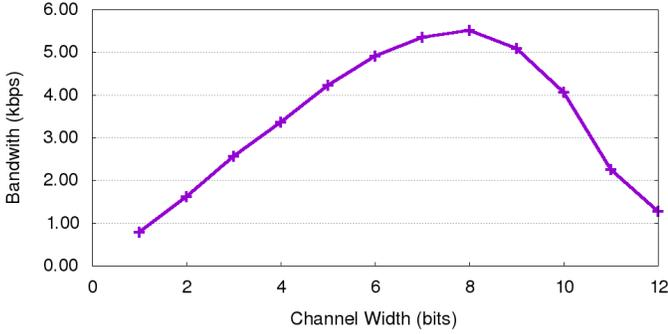
Fig. 8. **Speculative Bandwidth**—Using our speculative primitive, 1KB of data can be decrypted and exfiltrated at a speed of 5.38 Kbps from the speculative world with 20 redundant iterations per round (to ensure correctness). Increased channel width exfiltrates more data per round, but takes longer to measure the cache side channel. Optimal throughput is achieved with an 8-bit channel.
